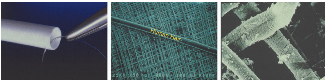
FIG. 2. Spun polyurethane vascular graft (left). SEM of fibrous vascular graft in comparison with a human hair (center) and unintended degradation of the polyurethane fibers comprising the vascular graft at 1-month postoperative (right). SEM, scanning electron micrograph.
